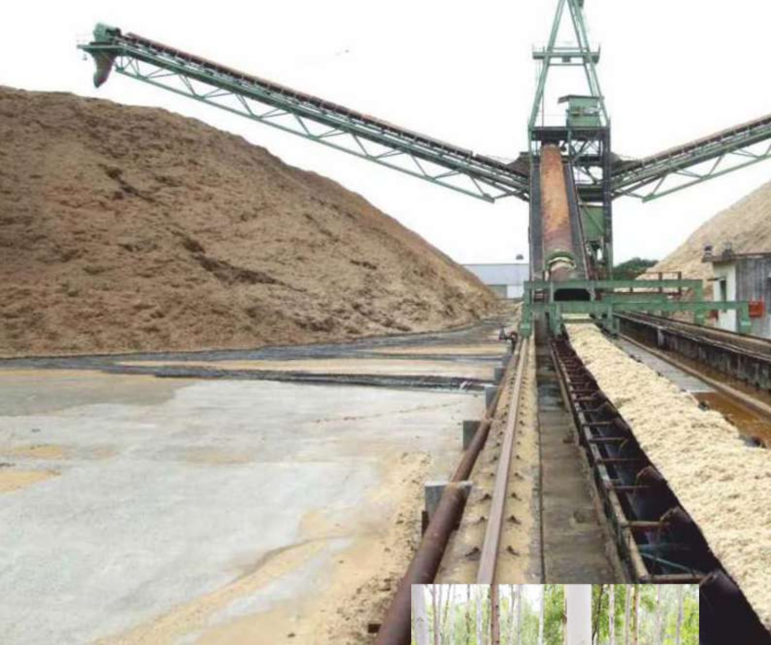
Stacker in Bagasse Yard, Unit-1
